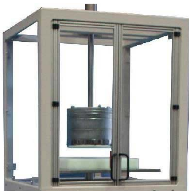
带砝码的压头，试样和支撑板
